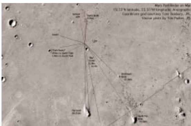
Figure B: NASA determined the location of the landing site by triangulating to known surface features.
